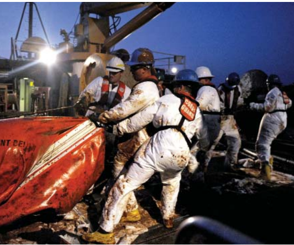
GULF OF MEXICO – Crew members from U.S. Coast Guard Cutter Harry Claiborne remove an oil covered boom that was part of a Vessel of Opportunity Skimming System. Photo courtesy of the U.S. Navy
