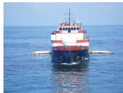
HOUMA, La. – A sweeping arm skimming system fitted on a commercial vessel collects oil in the Gulf of Mexico. Photo courtesy of U.S. Coast Guard
