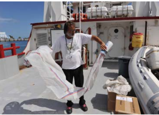
KEY WEST, Fla. – A staff member from the Florida Department of Environmental Protection demonstrates how the Neuston net is one of the mechanisms being used to monitor for oil from the Deepwater Horizon oil spill. Photo courtesy of U.S. Coast Guard
