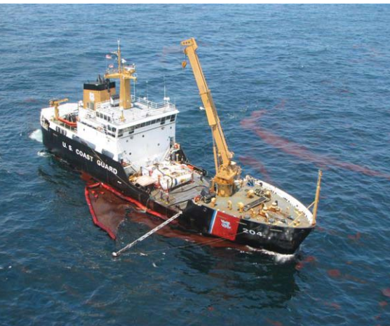
GULF OF MEXICO – Oil is collected in skimming boom attached to the U.S. Coast Guard Cutter Elm operating approximately 21 miles off the coast of Perdido Key, Fla. Photo courtesy of U.S. Coast Guard
