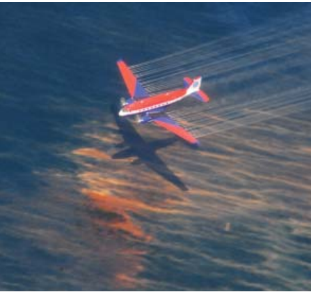
HOUMA, La. – The crew of a Basler BT-67 fixed wing aircraft release oil dispersant over an oil slick off the coast of Louisiana. Photo courtesy of U.S. Coast Guard.
